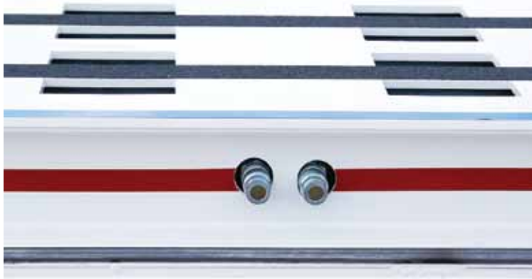
Quick connect hydraulic couplers, five each side, ten total.
