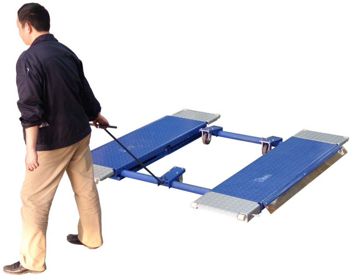
MOVING THE LIFT
