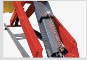
Mechanical lock and air-driven safety release.
